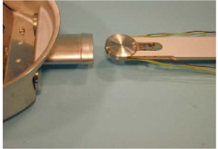
B. Insert the buffer tubes through the multiple cable port. If there is a number of buffer tubes, repeat insertion.
